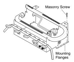
Figure 11 - Attaching Base Assembly to Fireplace Floor
